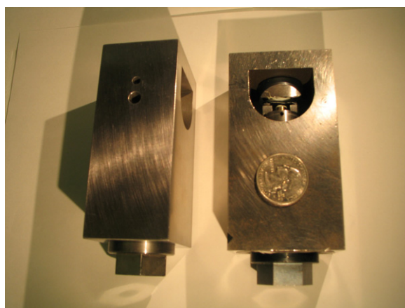
Figure 3. Magic-angle diamond-anvil cell.
